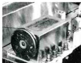
New Scott silver-plated four-nuovistor front end outperforms even the best conventional vacuum tube front ends. Nuovistors provide greater reliability, longer life, and guaranteed stability over years of use.
