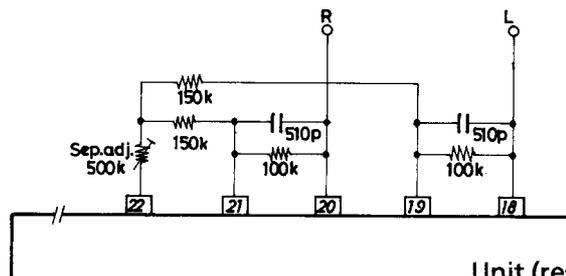
Unit (resistance:  $\Omega$ , capacitance: F)
