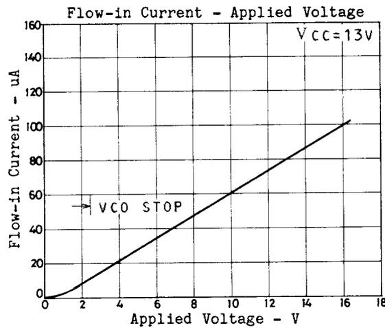
Fig. 1. Voltage Applied to pins 10, 26 – Flow-in Current
